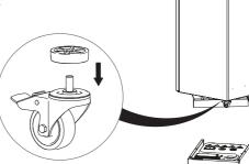
6 With at least 2 people supporting the appliance, using the 19mm socket, secure the front castors. It should be ensured that the castor spacers provided are fitted as indicated between the appliance base and the castor.
