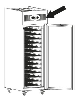
Regular cleaning of the condenser (located behind the front cover) increases energy efficiency and prolongs the life of your appliance.
