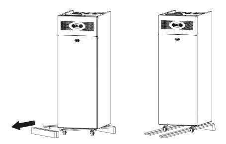
8 With at least 3 people supporting the appliance remove the rear section of the pallet as shown using the crow bar and hammer.
