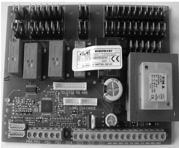
**Main PCB Front Display Connections**
