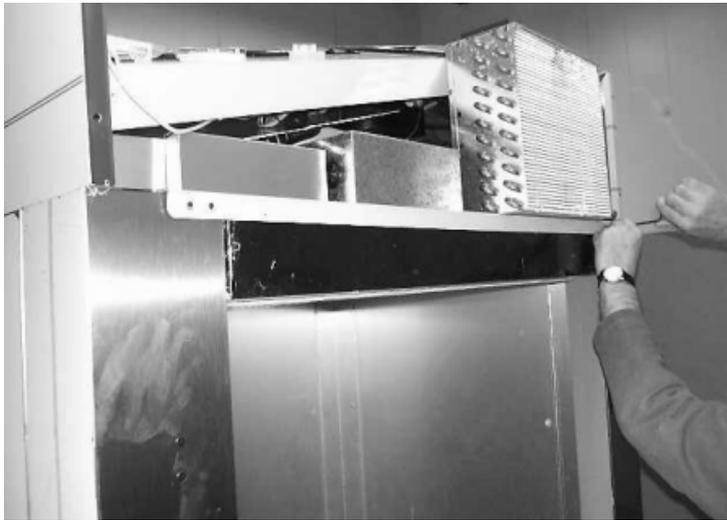
Fit the stainless steel angle brace that ties the 2 corners together using 2x M6 button headed socket screws ensuring that they are pulled square.
