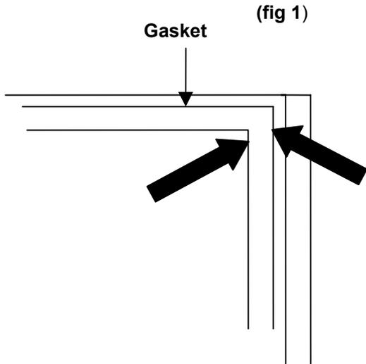
1. Using a sharp bladed knife make an incision in the soft part of the gasket in the top corner on the inner and outer. (See fig 1).
