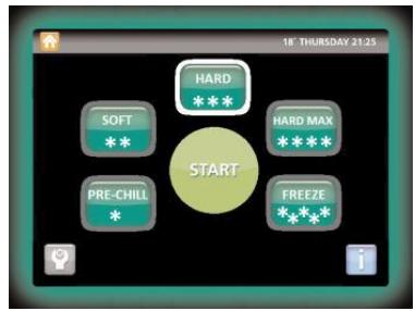
This is shown after initialisation and when no programmes are running. From this page a cycle can be launched. Select the cycle type by pressing the relevant cycle button and then press 'Start'. This page also shows the date, time and current air temperature and allows access to the 'Settings Home Screen' and 'Information' function.
