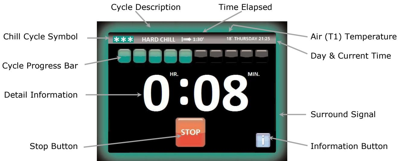
(Some icons or switches are only visible during adjustment, when activated by parameters or through operation/manual selection).
