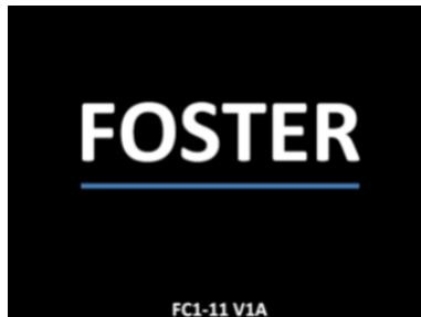
After power is applied to the unit the controller display will show the initialisation screen. This will only show for a few minutes stating both 'Booting' and then displaying the software version at the bottom of the screen. When the controller has completed initialisation the screen will revert to the 'Home Screen'.
