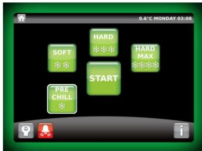
To view this alarm and or the alarm history press the flashing red alarm bell (as seen above) or if the alarm has been rectified access this history screen by navigating through the 'Service Settings' Screen and selecting 'Alarms'.
