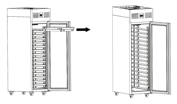
2 Release the level latch at the base of the rack.
