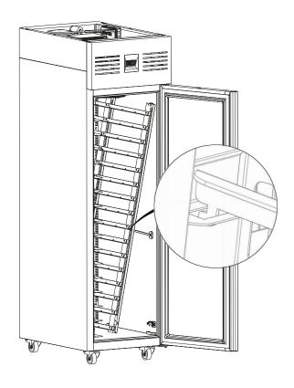
4 Refitting is the reverse of removal. Ensure that the lever latch is placed in the locked postion.
