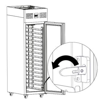
**3** Hinge the rack outwards and secure with the locking lever.
