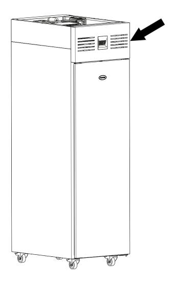
Regular cleaning of the condenser (located behind the front cover) increases energy efficiency and prolongs the life of your appliance.
