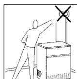
**9** The water shut-off valve must be within hand reach of the installed machine.
