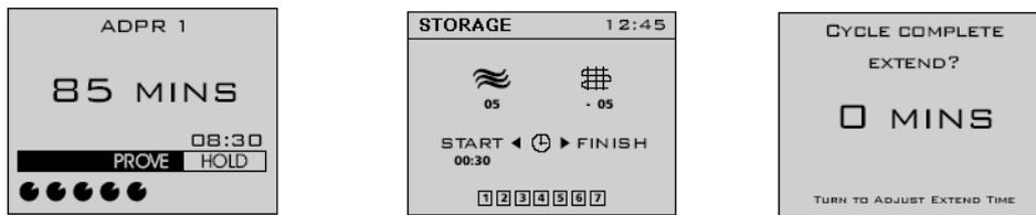
The screen will change to display the unit in 'RETARDING' mode, below left, with the temperature being displayed and 'HOLD' highlighted. The refrigeration system will lower the temperature until it reaches the storage setpoint when the screen will change to display 'STORAGE', below right. The controller will continue to operate within the storage temperature limits indefinitely initiating a time based defrost at pre-set intervals
