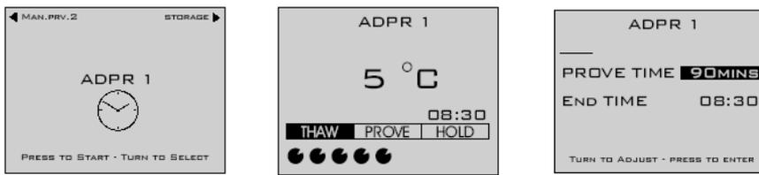
The controller will continue to control the temperature in the thaw mode until the time is reached for the prove cycle to start, below left. To achieve this the controller calculates back from the end time to determine the prove start time. Rotating the dial at any time will change the screen to display air temperature, evaporator temperature and the time that the programme has been running, below middle.
