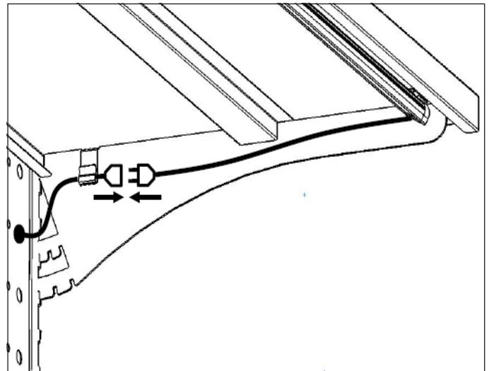
Plug the LED into the clipped cable tree branches.
